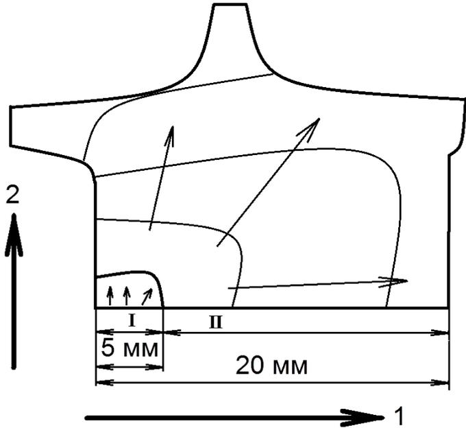
NUMBER OF CYCLES HAS BEEN DETERMINED BASED ON FATIGUE STRIATIONS COUNTING
