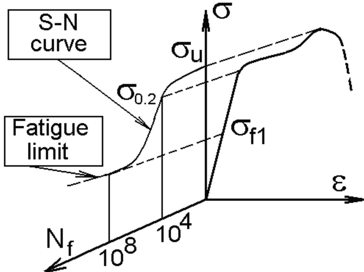
The cascade (a) of bifurcation transitions in behaviour of evaluated an open synergetic systems is describing as «Kelly's tree», and (b) the schema of the cascade of changes in behaviour of metals in process of increase of cyclic stress level.
