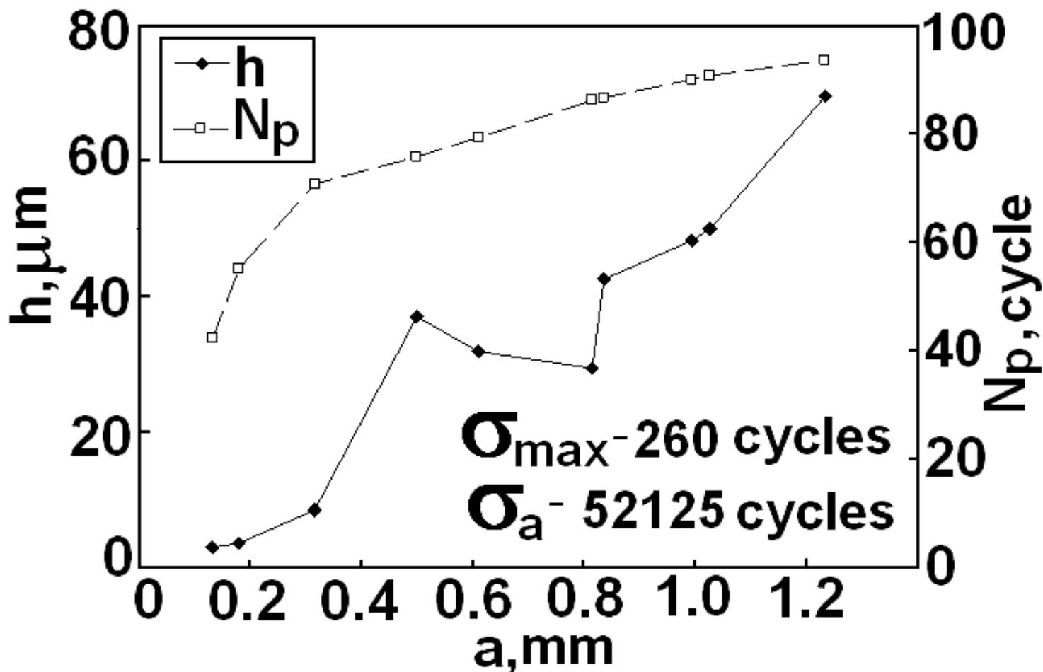
RESULTS OF SPECIMENS FATIGUE TEST AND FRACTOGRAPHIC ANALYSES FOR THE TITANIUM DISK No2 (6100 FLIGHTS TO FAILURE)
