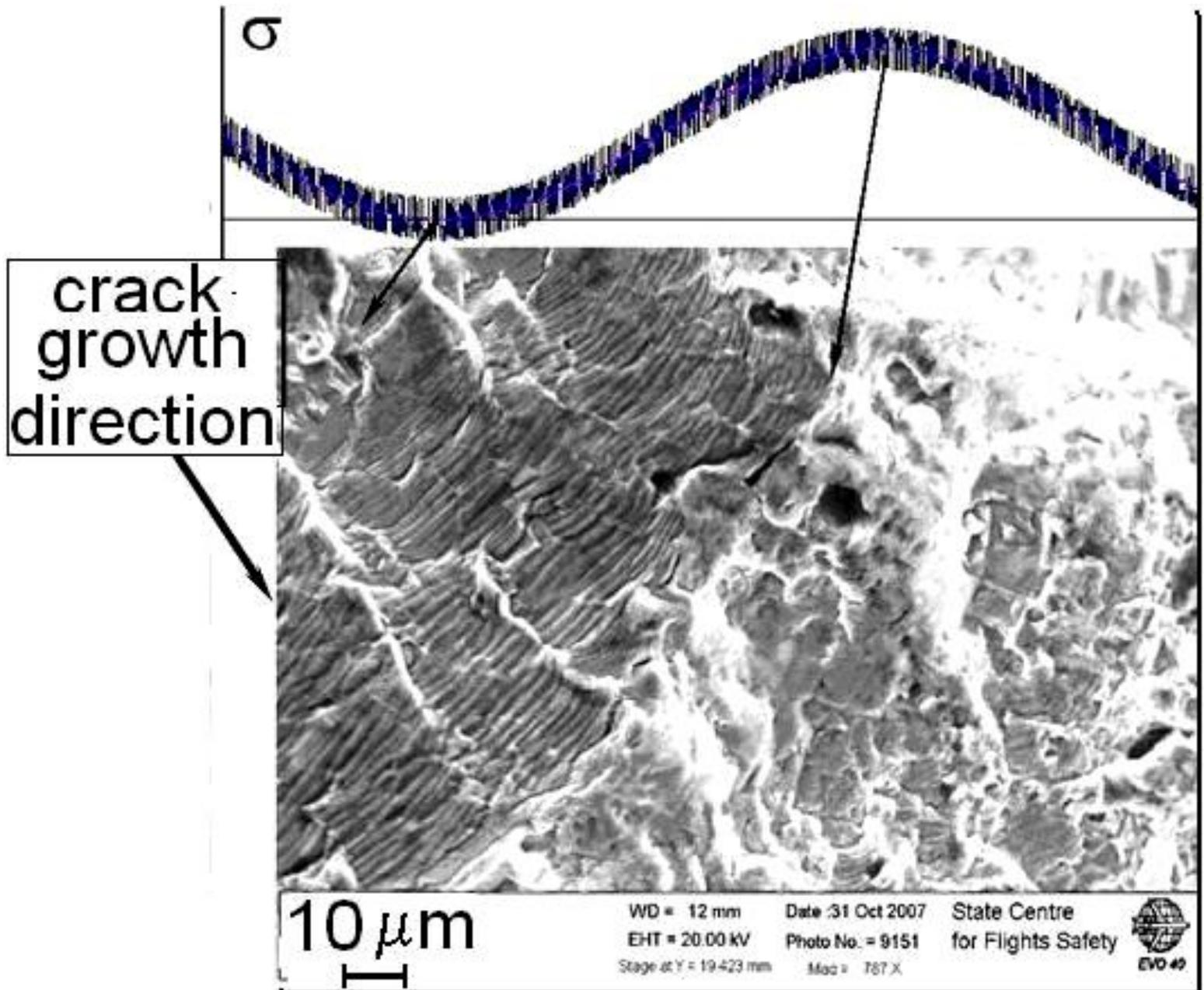
Fatigue crack increment during one block of cyclic loads versus crack growth length for the tested specimen under stresses  $\sigma_a = 210$  MPa and  $\sigma_{max} = 500$  MPa.
