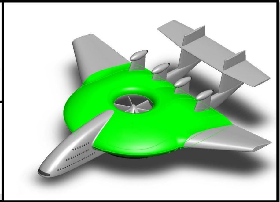
Fuselage for helium – volume: 6600 m<sup>3</sup>; lift: 6976 kg
