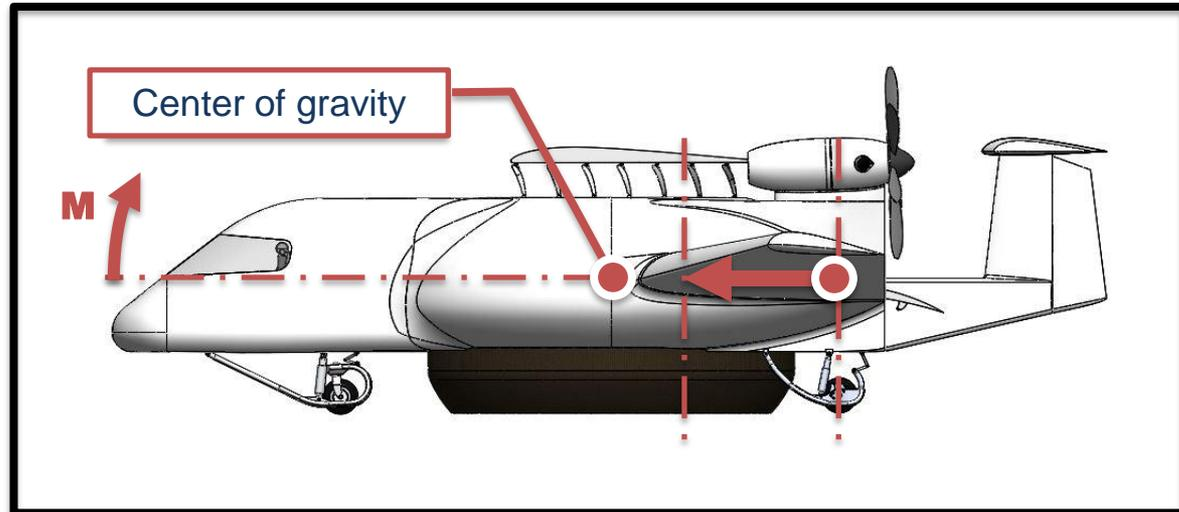
Placement of landing gears
