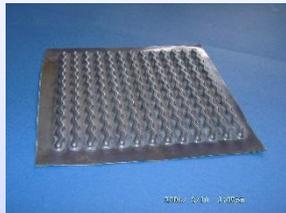
Wave structure for heat exchanger 1.4462, 0,15 mm
